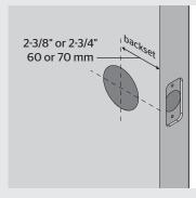
Measure to confirm that the hole in С the door edge is 1" (25 mm).
